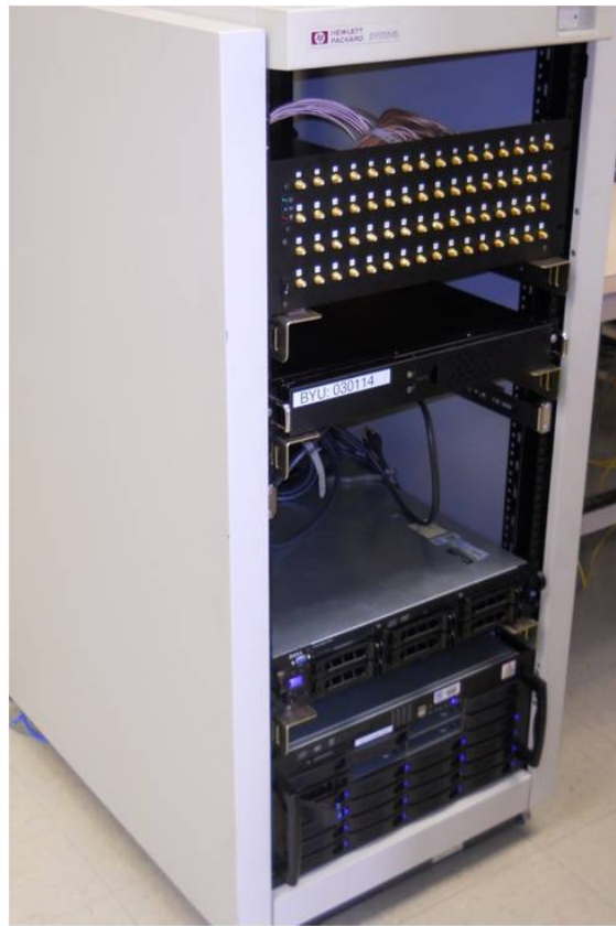
Figure 6.4: Equipment rack configuration with ROACH and 64 RF input connections for the x64adc (top), a second ROACH which will perform beamforming operations (middle) and host computers and data file server (bottom).
