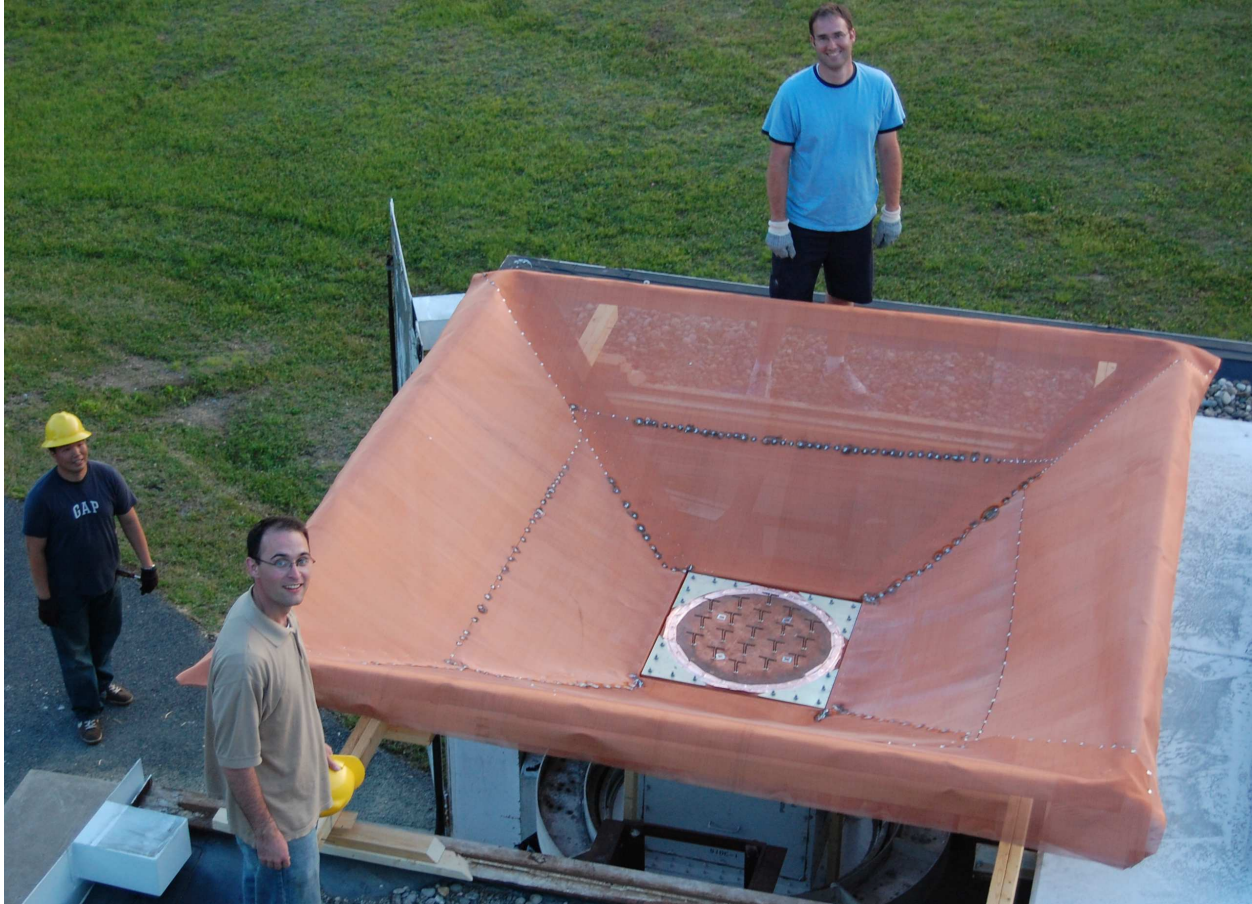
Figure 4.6: Overhead view of ground screen. The array is mounted on the FEB containing the front end receiver electronics, and the wood frame of the ground screen sits on the structure that holds the FEB in the outdoor test facility shown here. The copper screen is rounded around the edges of the wood frame to help reduce diffraction that would introduce interference from sources around the screen.
