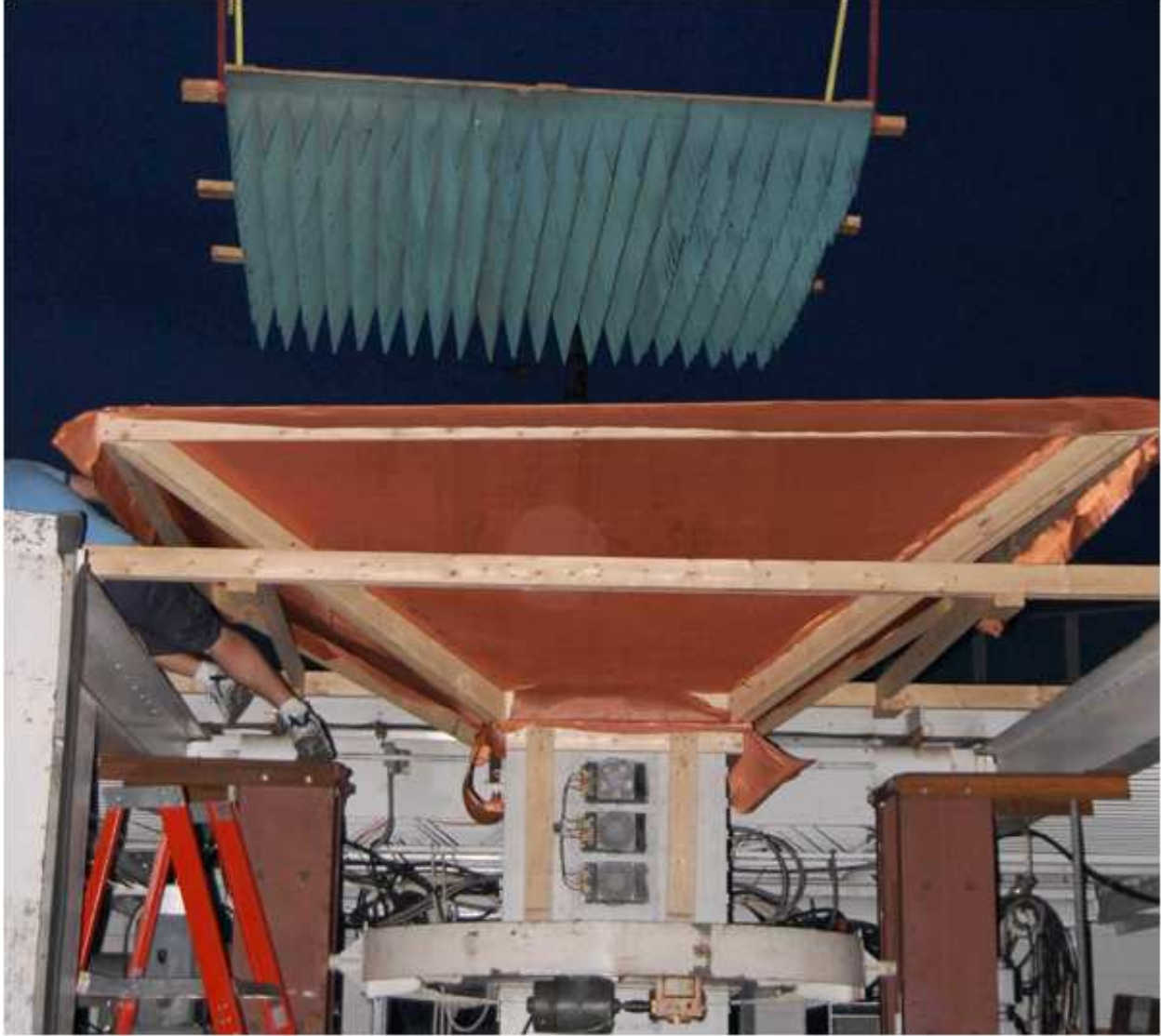
Figure 4.8: Absorber being lowered into the ground screen
